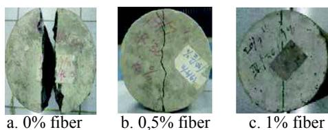
Figure 5. Mode of failure under splitting test
