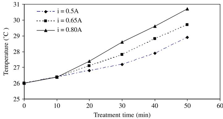
**Figure 4** Effect of treatment time on temperature
