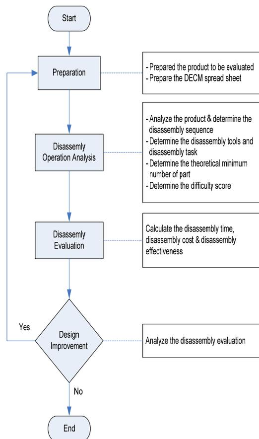
Figure 1: Disassembly evaluation chart procedure
